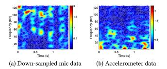
Figure 4: Spectrogram comparison between the accelerometer data and the down-sampled microphone data (illustrated with the command "show facebook.com").
