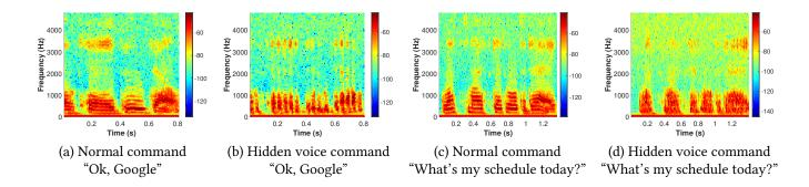
Figure 6: The power spectrum of the surface vibrations of normal commands and the corresponding hidden voice commands, as measured by a laser vibrometer pointed at the smartphone.
