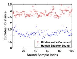
Figure 9: Euclidean-distances of the voice command samples to the human speaker sound cluster centroid based on vibration features.
