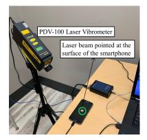
Figure 5: The experimental setup for surface vibration measurement using laser vibrometer.
