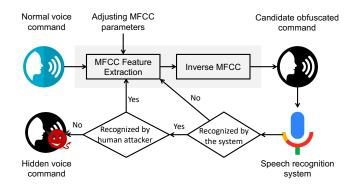
Figure 1: Workflow of generating hidden voice command [9] from a normal voice command.
