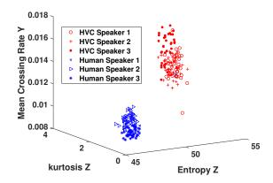
Figure 8: Illustration of the vibration features to distinguish hidden voice commands and normal commands.
